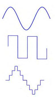
Sine Wave- This is the wave form of good clean utility power. More expensive to produce with a ups system.
